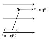
In non-uniform field both force and torque is non zero.
