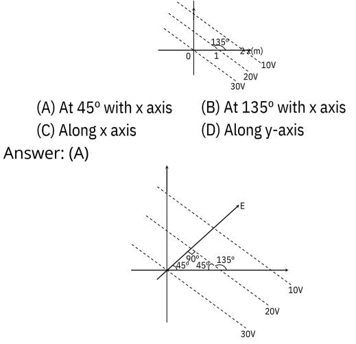
Electric field lines are  $\perp$  to the equipotential surface and are directed from high potential to low potential.
