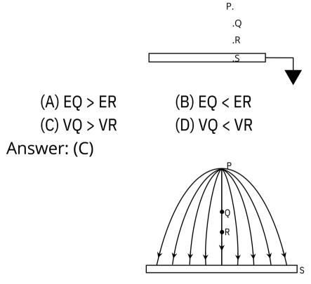
As we are are moving away from P toward sheet S spacing between electric lines of force is increasing.
