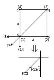
... Net force on charge q is F = F122 + F13 $= \frac{kg}{a_2}22 + \frac{kg}{(a\sqrt{2})2}$
